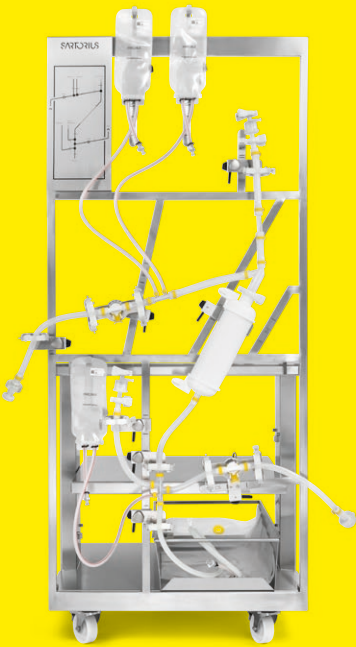
Figure 1: Stainless steel holder with filter transfer set final filling assembly.
